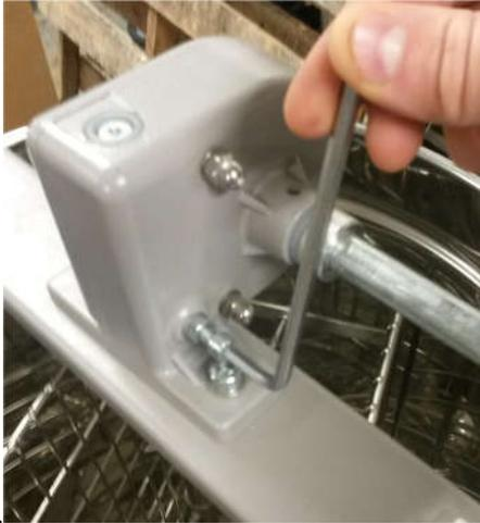
2. Remove the gearbox and crank from the top bar (4 bolts). Hang on to the gearbox in case you decide to use it again.
