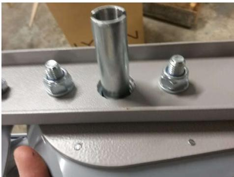
8. Reinstall the top bar on the extractor. Be sure to align the gearbox and the extractor shaft. On the right side, use the 8mm nut (included) in addition to the cap nut that was already part of your extractor (the stud is too tall otherwise).
