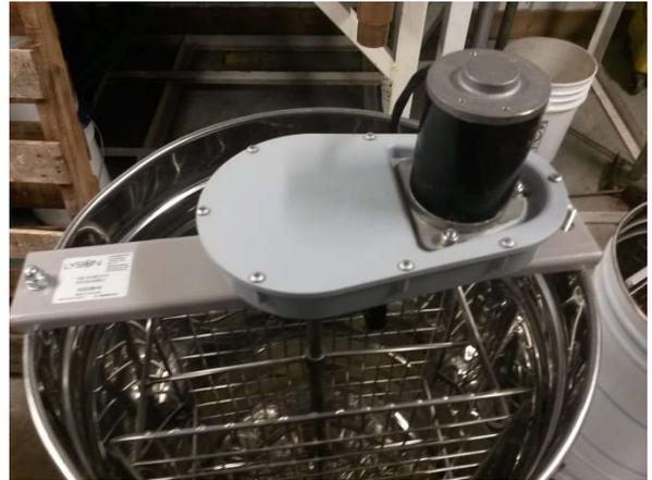
**Note:** for 12-frame models, you may need to move the hinges on the right side to the right to make room for the motor. Re-attach the hinges with ½ of the screws (see below).
