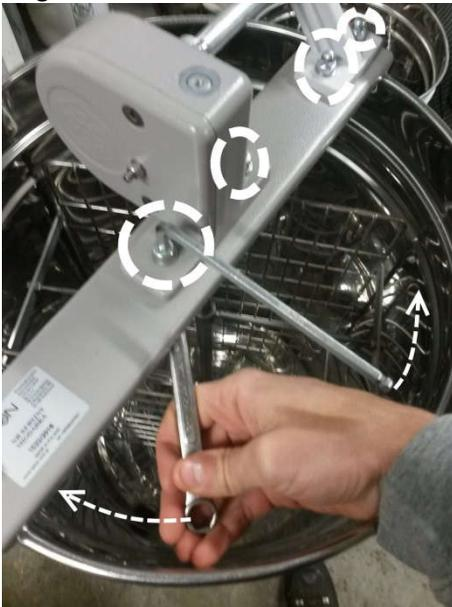
3. Temporarily place the motor on the top bar as shown below. There are two bolts that will align with holes in the top bar. Do not install the nuts yet.
