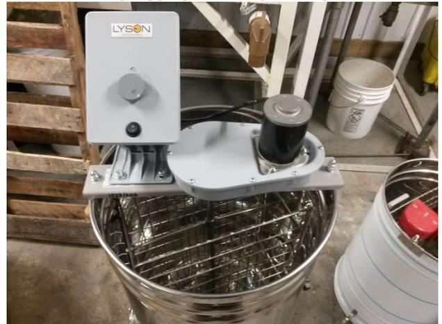
10. To operate extractor, turn knob to left (lowest speed). Then, turn the switch on to the "1" position. Gradually increase speed until the extractor spins.
