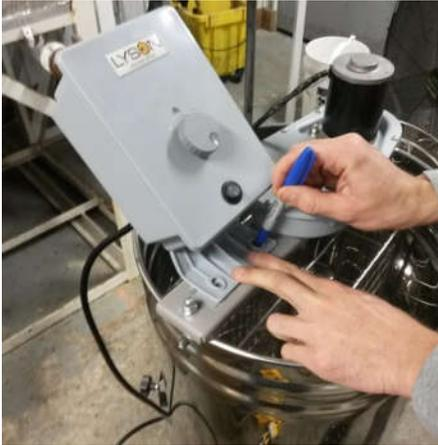
5. Remove the gearbox and controller. Then remove the gray top bar from the extractor.
