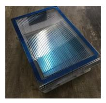
8 Place melter in a bright sunny level location on a warm day. Allow several hours for wax to start melting and check progress periodically. Change wax filled catch basins and clean metal pan of debris when needed. For large or heavy dirt batches, it may take more than one day to process the wax.
