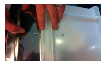
5. Rest metal pan on lip inside the metal rim, so that holes in the open end of the pan line up with holes in the plastic box. Thread the metal rod through the holes in the plastic box, metal pan, screen/baffle and through to the other side. This will act as a hinge when you insert the catch basin.
