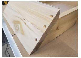
5. Install the remaining 2" screws in the back corners.
