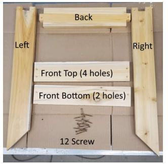
2. Assemble the Back to the Left and Right pieces with 2" screws. To start, use just one screw per corner.
