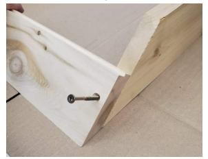
4. Install the Front Top board with 2" screws (the board with four screw holes).
